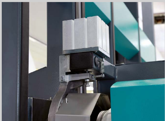
Pneumatic control of fixture
