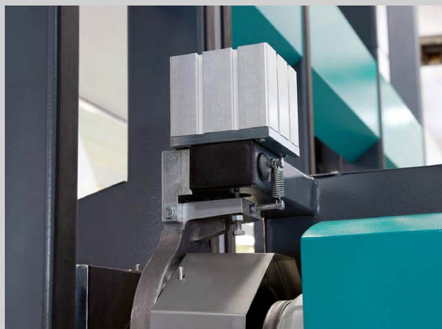
Pneumatic control of fixture
